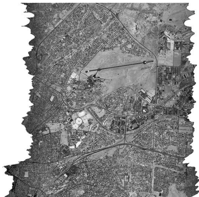
4200m wide single-pass swath acquired from 2800m AGL flying height, avg. point spacing: 1.6m
