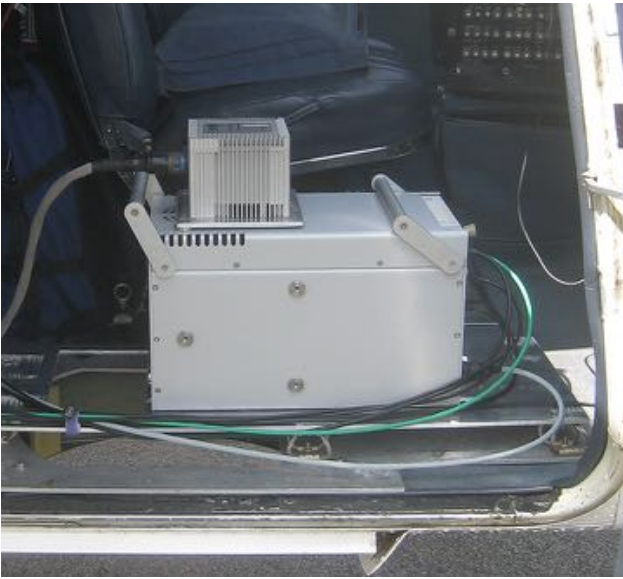
EL-MAP installation on Cessna 337
